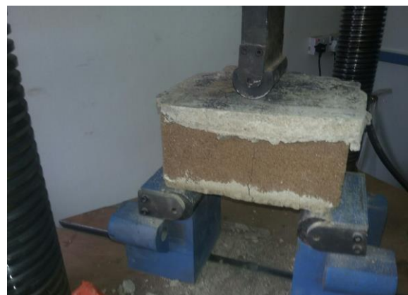
Plate 2.7: Flexural Test on Block Samples
