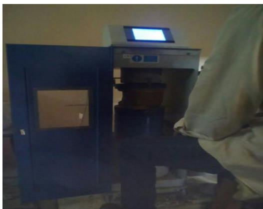
Plate 2.6: Compression Test on Block Samples
